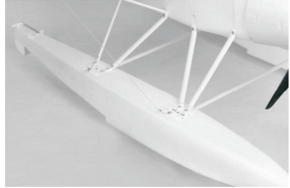
Mount the mid end of bracing robes to the wing struts and mount the other ends of bracing robes to the floats with M2.5x8 tapping screws. The holes that be mount bracing robes on each floats should be symmetrical.
