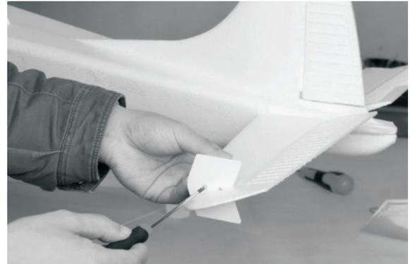
Ensure to bracing robes of both side are equi-long. You can ajust the length of bracing robes by tying or untying knots on it.
