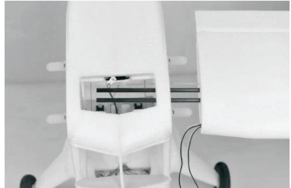
Remove the top hatch from the fuselage and mount the wing locker by M3.0x10 tapping screws.
