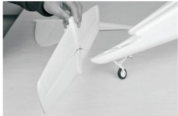
Pull the elevator pushrod wire a bit out of fuselage, then insert the „Z - bend“ of the wire into the bottom hole in the elevator horn as show.
