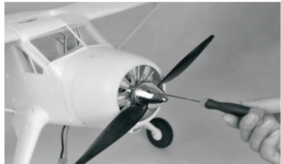
Insert the collet prop adapter through the prop hub.
