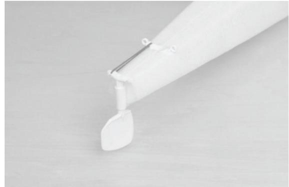
Pass the pull-thread of water rudder through a rubber band. Then hang the rubberband onto hook of float and water rubber arm as illustration. Do the same to the other water rudder.
