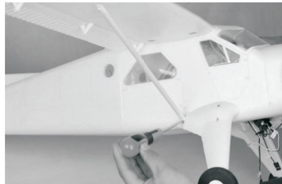
Put the end A onto the retral hole of landing gear, then insert the spared tapping screw.
