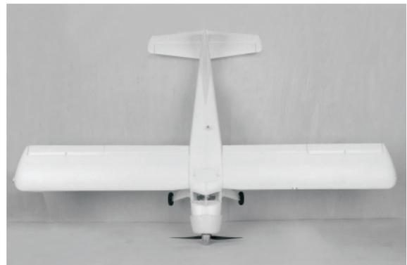
Install the motor battery, but do not connect it to the ESC. Also install the battery hatch. All the rest of the parts of landing gear version model should already be installed.
